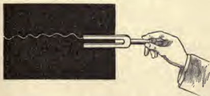
FIG. 129. — The Motion in the Prong of a Fork is Vibratory.
